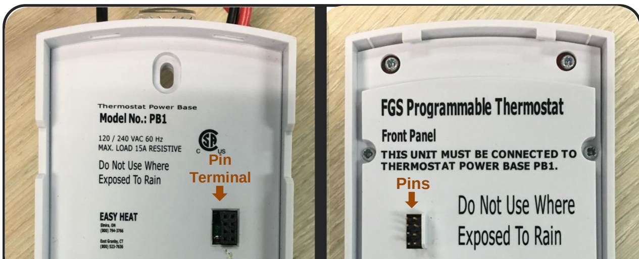
Figure 2: FGS Thermostat Power Base (PB1) and Front Panel
